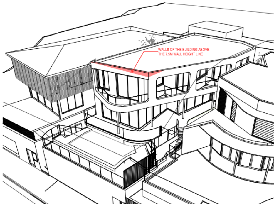
Figure 5: Three-dimensional plan showing area of wall height non-compliance
