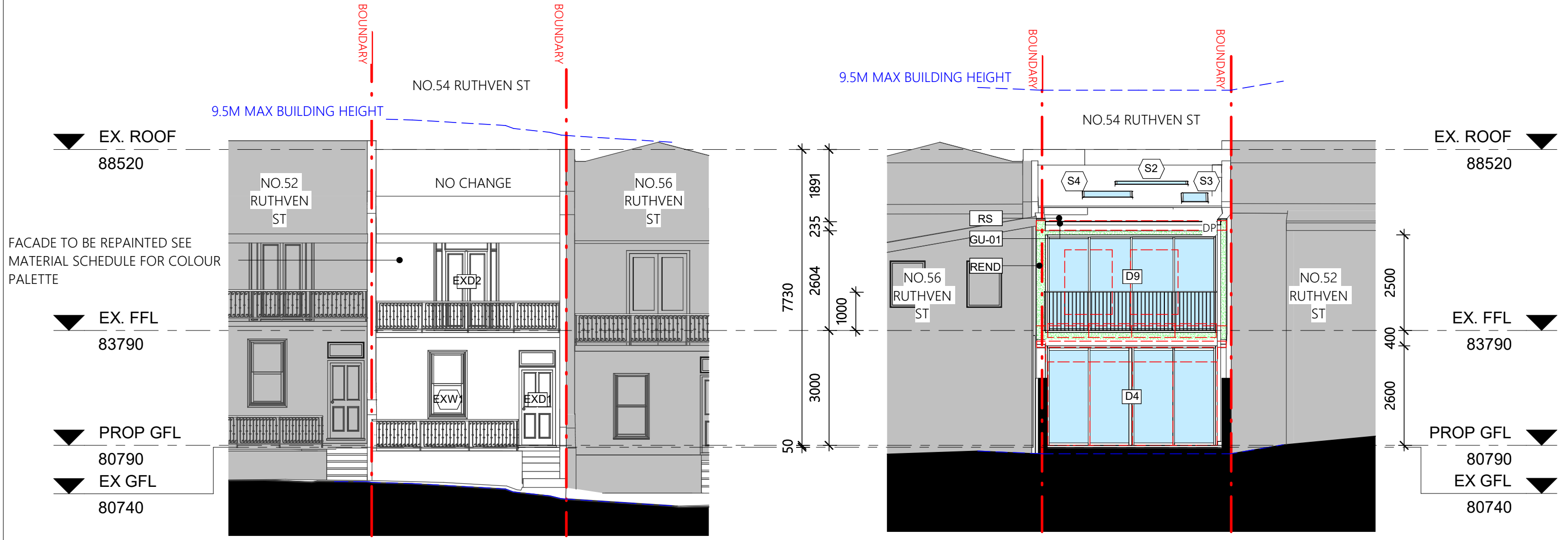
1 WEST - STREET ELEVATION (NO CHANGE) DA200 1:100
