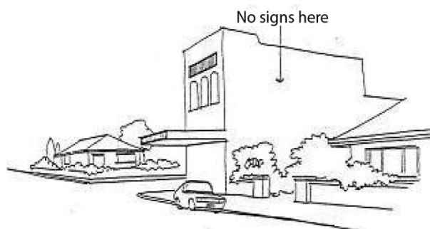
Figure 29 Inappropriate location for flush wall signs
