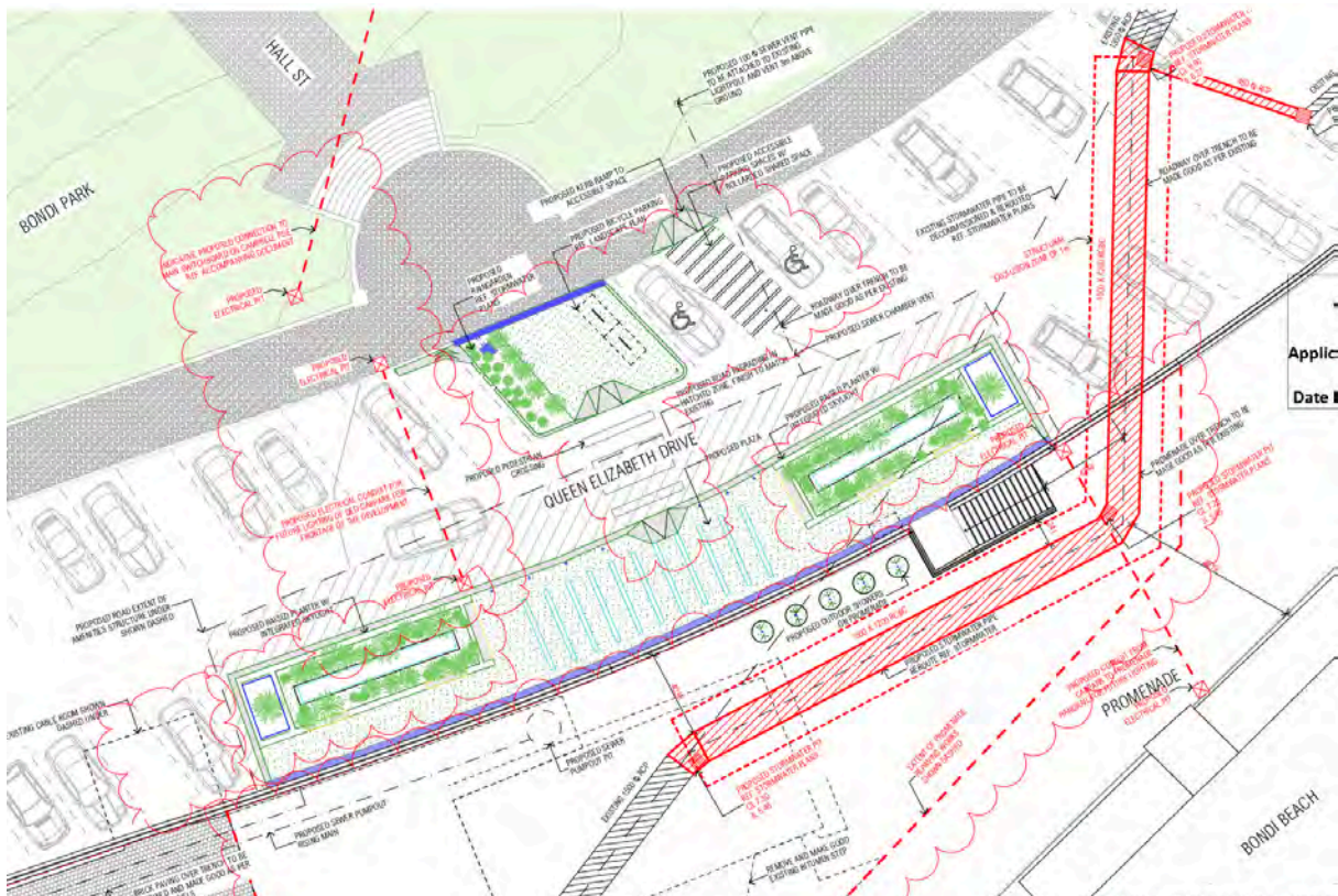
Figure 7.22: Roof plan / QED road plan for the Southern Amenities showing the proposed platforms and skylights / planters. The toilets and small kiosk are under this. The red clouds indicate where the design was changed from the initial DA drawings. The red hatched dogleg area on the right is the diverted stormwater drain. Source: DA Waverley Council website
