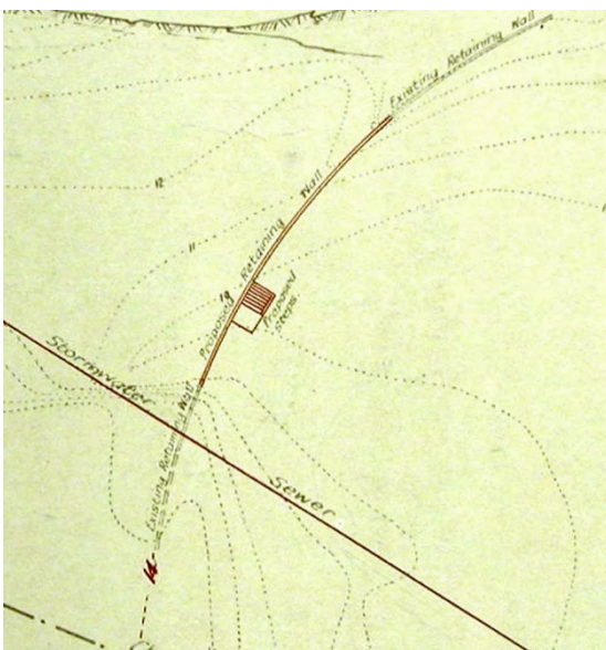
Figure 5.48: Part of a mid 1920s plan for Tamarama shows a proposed sea wall joining two sections of existing wall, with steps to the sand from a new promenade. Source: WLS photograph of original
