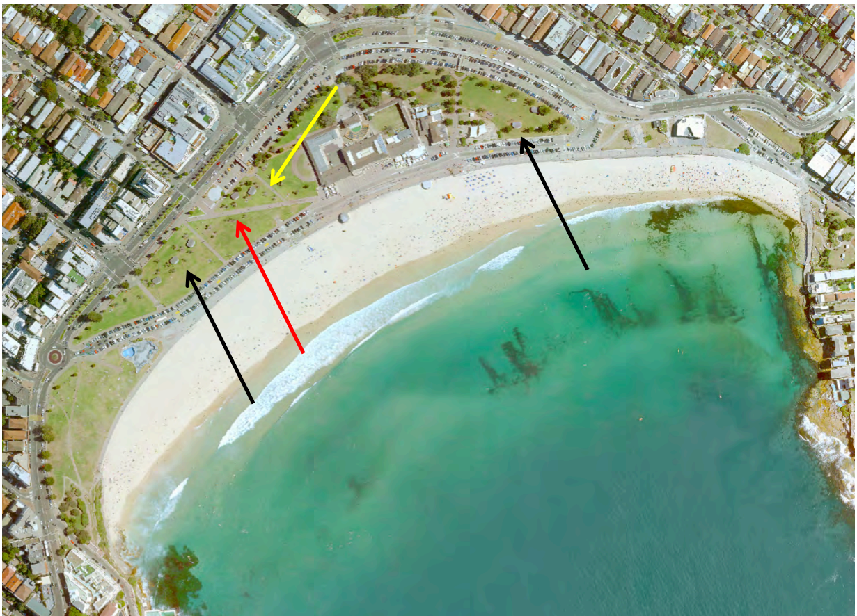
Figure 4.76: 2018 aerial photo. New wide diagonal brick path added (red arrow). New path in similar location to former but level is raised and does not continue to QED (arrowed yellow). The new picnic shelters are also shown in this image as grey rectangular forms, 5 on the mid slopes south of the pavilion and 2 to the north (black arrows) Source: Waverley Council
