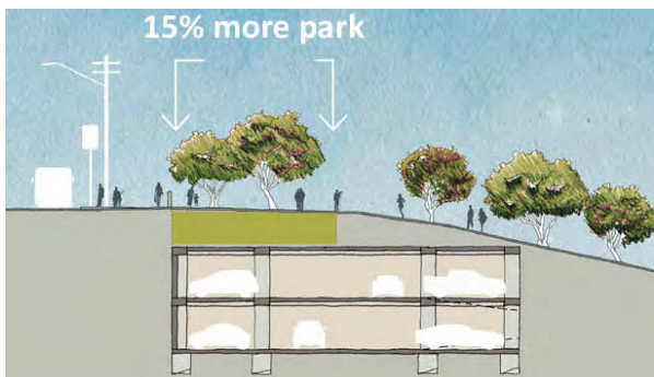
Figure 7.13: Extract from above showing the proposed underground carpark. This has been removed in the 2021 update. Source: Waverley Council
