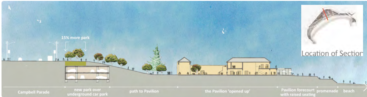
Figure 7.12: Cross Section from 2014 Master Plan showing the then proposed underground carpark. The green area over the underground carpark indicates the existing Motor Drive that would be removed. Note that the proposed carpark is about double the width of the existing and the lowest floor would be about 8m below Campbell Parade with footings below that. The underground carpark and greenspace has been removed from this section in the 2021 update. Source: Waverley Council
