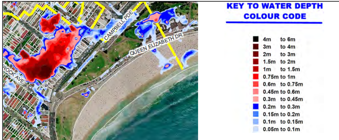
Figure 4.15 Approximate Extent of Overland flows in 100 year ARI Event (Source: Civic Design, 2007)
