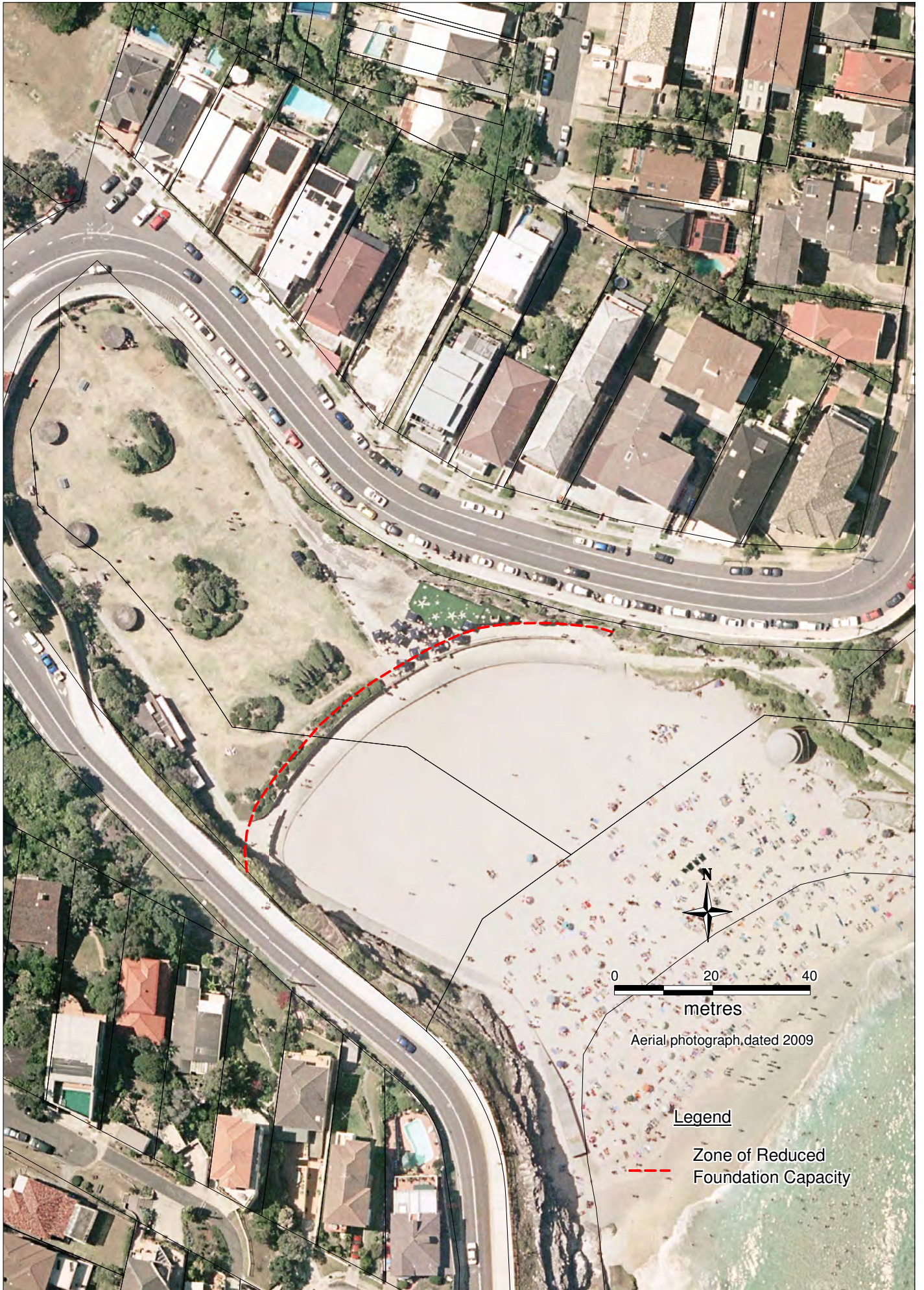
ZONE OF REDUCED FOUNDATION CAPACITY AT TAMARAMA
