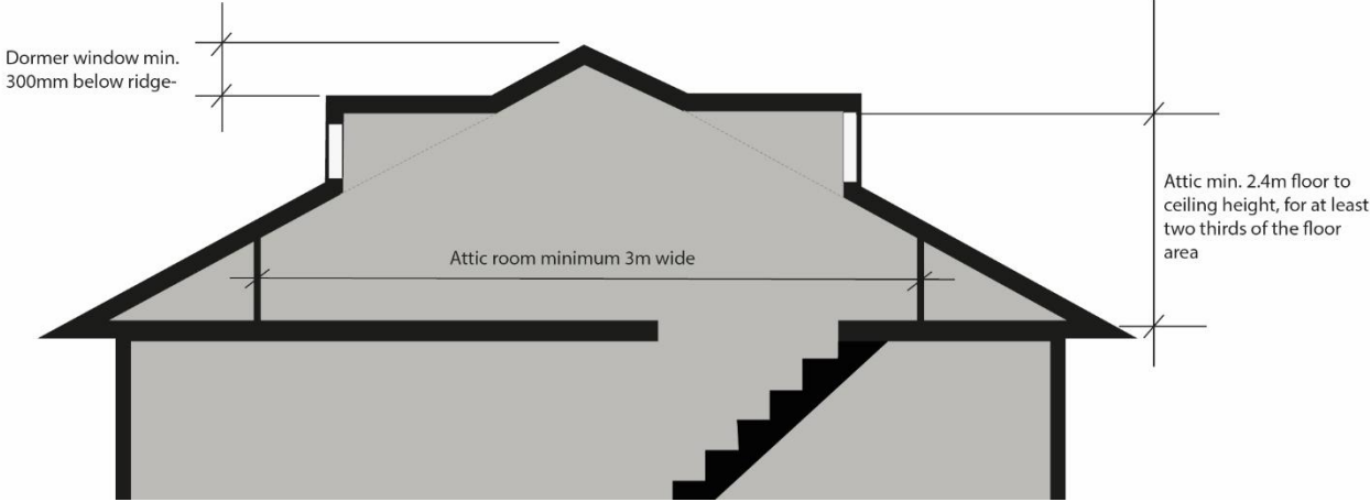
Figure 21 Pitched roof minimum attic dimensions
