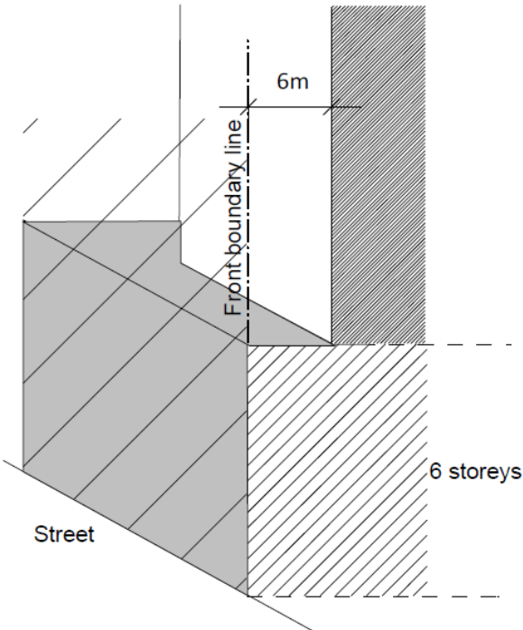
Figure 13 Setbacks from the street: buildings in street without heritage
