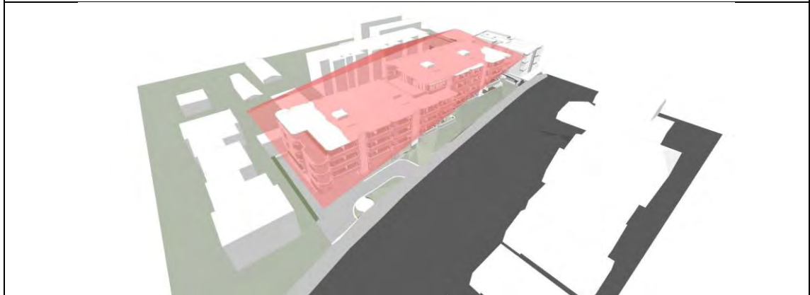
Figure 9: Height plane (view from the north west perspective) showing the areas of height non-compliance being the lift three of the four overruns, a portion of the south west corner and the northern parapet
